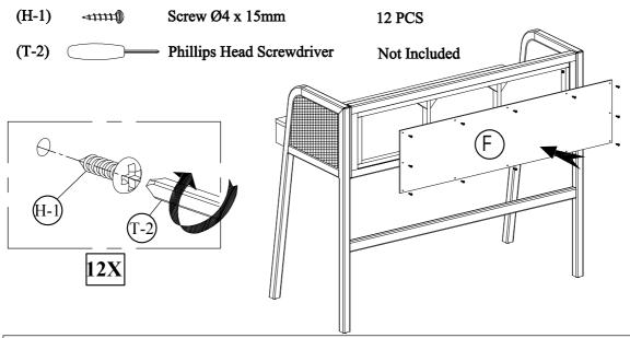
Using a second person to assist you, carefully set the assembly upright. Position and secure the Back Panel (F) to the Back Frame (D) by inserting Screws (H-1) into the pre-drilled holes and tightening using Phillips Head Screwdriver (T-2; not included). Do not use a power drill and do not over tighten, as doing so might cause damage.
