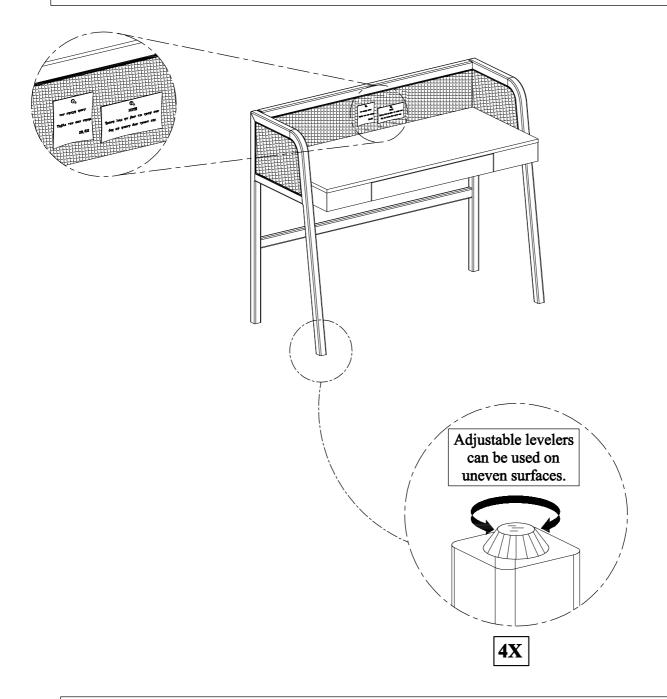
Ensure that all bolts have been fully tightened. Assembly is now complete and the table is ready for use. NOTE: Check that all bolts remained fully tightened every 3 months to ensure stability.
