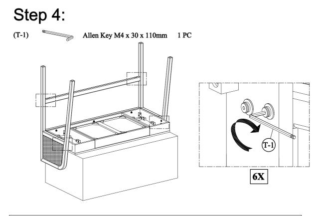
Using the provided Allen Key (T-1) fully tighten all bolts from previous steps. Do not over tighten.
